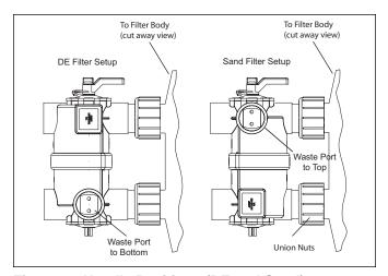
Figure 1. Handle Positions (DE and Sand)
