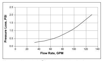
Figure 6. NeverLube® Backwash Valve Performance Curve
