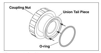
Figure 2. O-ring Placement
