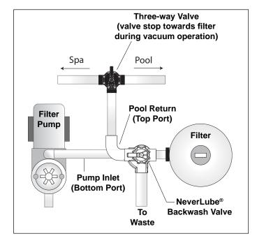
Figure 5. Vacuuming to Waste
