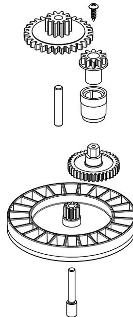
Medium Turbine/Spindle Gear Kit
