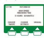
If the motor does not start in High Speed, the user may need to select Manual, then start on High in order to prime the pump.
