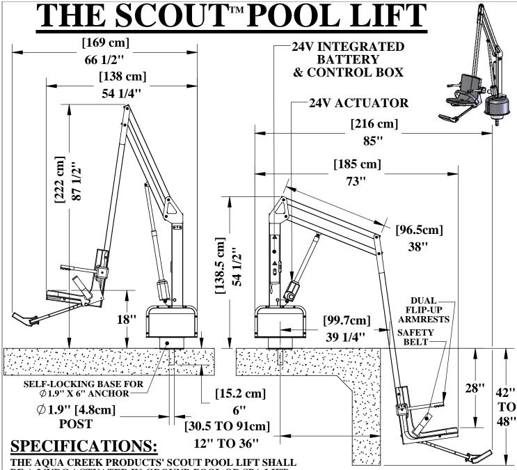
BE A 24VDC ACTUATED IN-GROUND POOL OR SPA LIFT.
