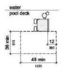
4. Submerged Depth. The lift shall be designed so that the seat will submerge to a water depth of 18 inches (455 mm) minimum below the stationary water level. To make sure the lift has enough clearance the lift should be installed at a location with 48" of Water depth
