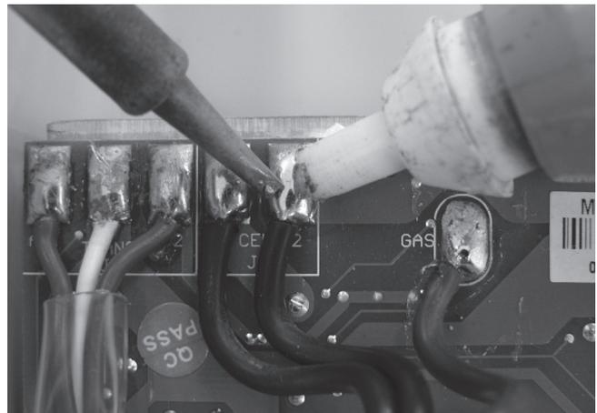
**Step 4** – With a soldering iron & solder sucker or solder wick remove the wires for the cell cables & gas sensor. When the metal has cooled remove the cell cords.
