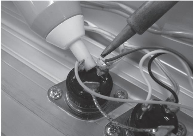
**Step 1** – Using a soldering iron & a solder sucker remove the wires connected to the Triacs. Mark the positioning of the wires to assist in reconnection.
