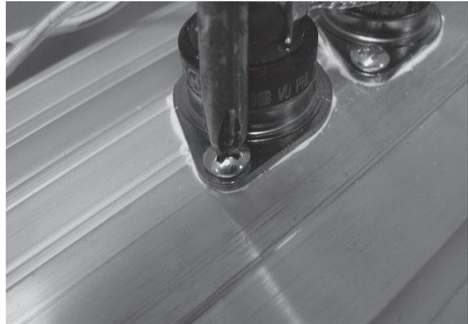
**Step 2** – Remove the screws connecting the Triacs to the chlorinator using a Phillips head screwdriver (two point) & remove the Triacs.
