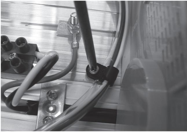
**Step 3** – Feed the secondary transformer wires through the clear tubing then using the wire clamp, fasten the wires back onto the chlorinator using a Phillips head screwdriver (two point).
