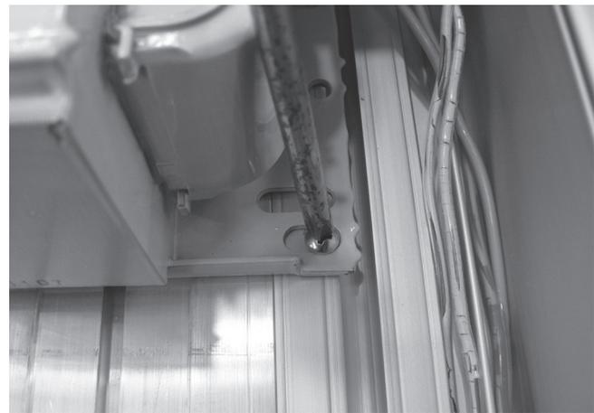
**Step 4** – Remove the screws holding the transformer in place using a Phillips head screwdriver (two point).
