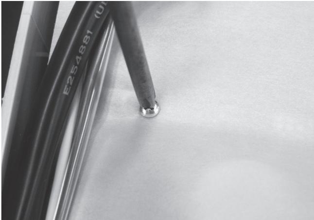
**Step 1** – Remove the screws holding the cover on the PCB with a Phillips head screwdriver (one point).
