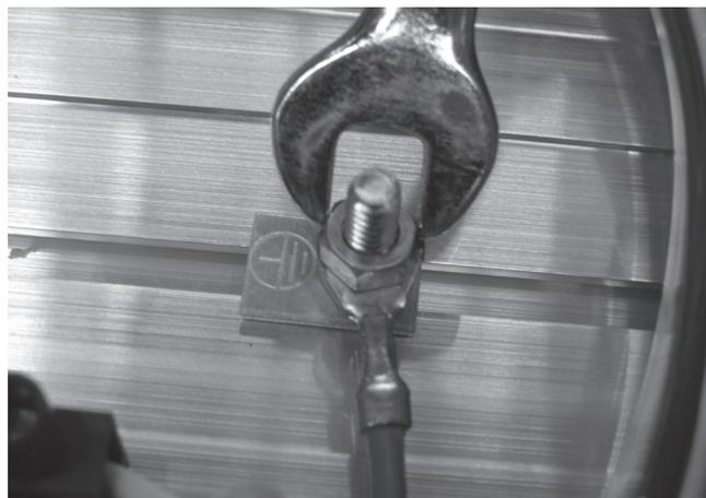
**Step 2** – Remove the nut holding down the green Earth lead using an 8mm spanner.
