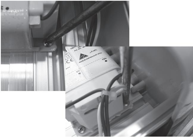
**Step 5** – Remove the locating screws connecting the transformer to the chlorinator. Remove the front two first using a Phillips head screwdriver (two point) then using a long blade Phillips head screwdriver remove the rear screw.
