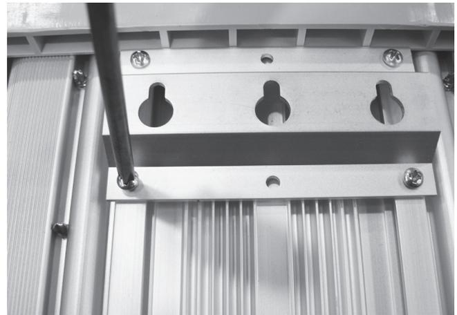
**Step 1** – Place hanging bracket in position over screw holes & replace screws using a Phillips head screwdriver (two point).
