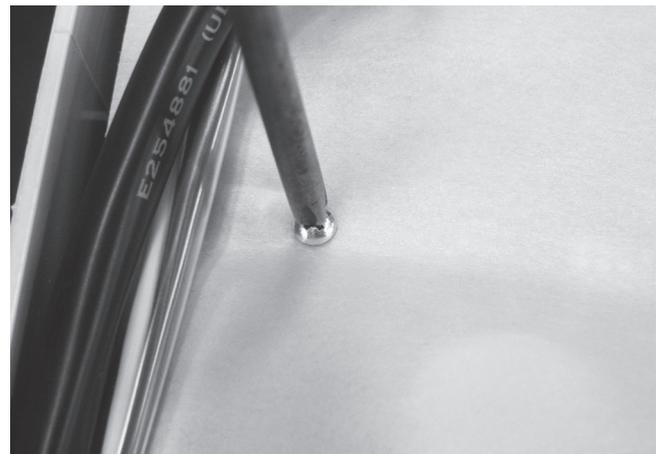
**Step 4** – Remove the screws holding the protective covering on the PCB using a Phillips head screw driver (one point).
