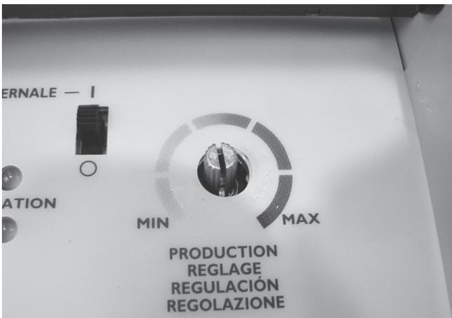
**Step 3** – When PCB is in place the sanitiser output holder will be visible poking through the front panelling. Reconnect sanitiser output knob to its holder ensuring it is able to be adjusted to both minimum & maximum settings.
