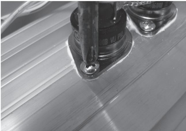
**Step 1** – When placing the Triacs back onto the chlorinator use a heat transfer compound such as Unick to assist with heat dispersion during operation. Unick is generally available from electrical repair stores & some electronic retailers. Fasten the Triacs down using a Phillips head screwdriver (two point).
