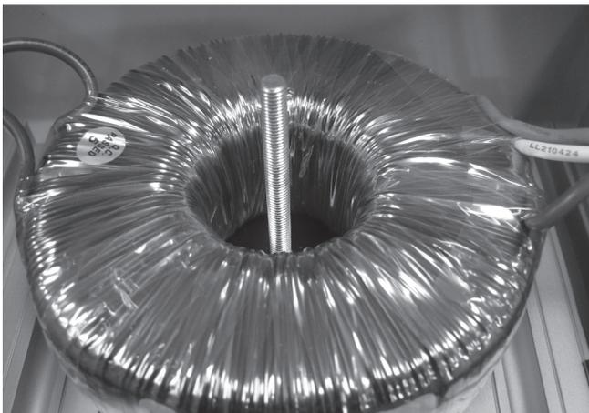
**Step 1** – Place transformer over the locating screw.
