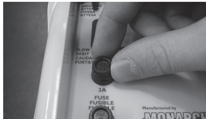
**Step 2** – Place fuse into fuse housing & pushing gently down twist to the right to lock in place.
