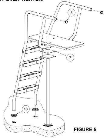
5. Place **Gasket (item 7)** onto footboard and align holes to each other. Place **Swivel Stand W/ Umbrella Holder (item 4)** onto gasket and align holes to each other. Place and hold
