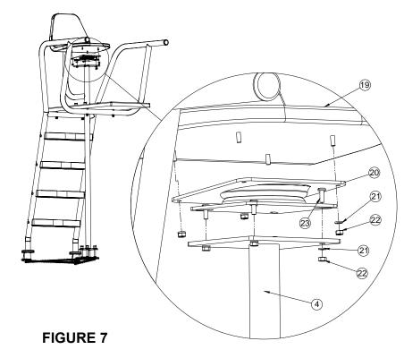
as shown in FIGURE 7. Tighten hex nuts.
