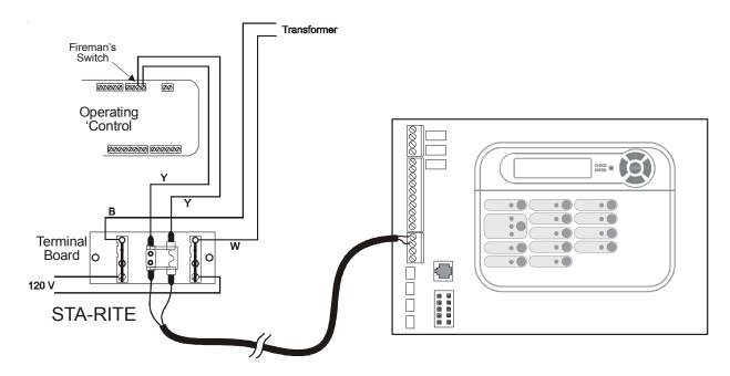
**Hayward Variable Speed Filter Pump:** Refer to the diagram below for proper low voltage communication wiring between the Pro Logic and the Hayward Tristar Variable Speed Control (VSC).
