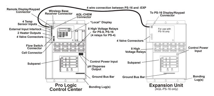
The Pro Logic Control Center and PS-16 Expansion Unit require both high and low voltage connections. Low voltage connections will be made to actuators, sensors, remote keypad, etc. High voltage connections will be made to pumps, lights, etc., as well as providing direct input power to the Control Center. Always:
