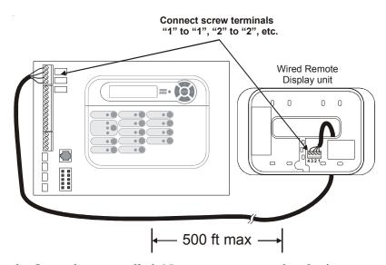
If multiple remote display/keypads are installed: Never connect more than 2 wires to any terminal block. Two remotes can be wired back to the Pro Logic main unit or the second display/keypad (and third, if applicable) can be "daisy chained" with one display/keypad wired to the next. The maximum wire run from the Pro Logic main unit to the furthest remote display/keypad is 500 ft (160m).
