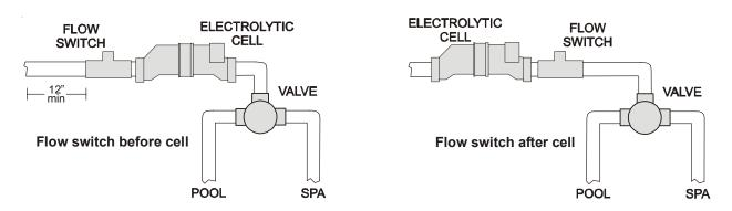
The cell may be mounted vertically or horizontally, and water can move in either direction through the cell. Install using the 2" unions provided in the P-KIT purchased separately. Tighten unions **BY HAND** for a watertight seal. For systems with 1½" plumbing use adaptors (provided by installer).
