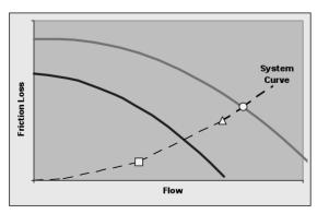
In this example, the flow for the 3/4 HP pump is between the minimum and maximum flow and is therefore properly sized for the application.
