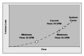
The point where the performance curve for a particular pump intersects the system curve determines the flow and Total Dynamic Head where that pump will operate.
