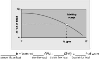
Choose the minimum and maximum flow rates based on Turnover Rate and Water Velocity and calculate the corresponding friction loss using the formula
