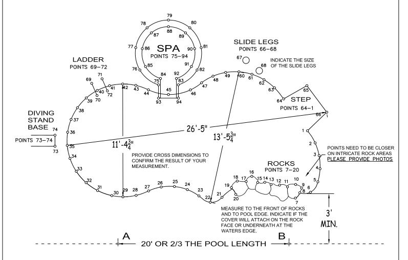
NOTE: MAKE SURE THE A-B LINE IF EXTENDED IS NOT CROSSING THE PERIMETER OF THE POOL.
