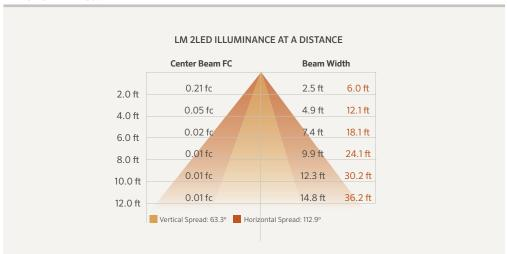
Beam angle is calculated using LM-79 method for SSL Luminaires:
