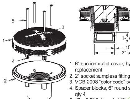
**6" Bulkhead Adapter with 2" Threaded x 1 1/2" Socket Sumpless Fitting (sold separately)**
