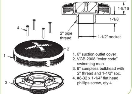
**6" Bulkhead Adapter with 2 1/2" Threaded x 2" Socket Sumpless Fitting (sold separately)**
