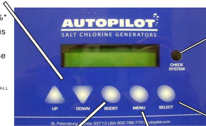
**CHECK SYSTEM** – Red LED flashes to warn attention is required. A warning message will also be displayed. If enabled, an audible alarm\* may also be heard when the system light is flashing.
