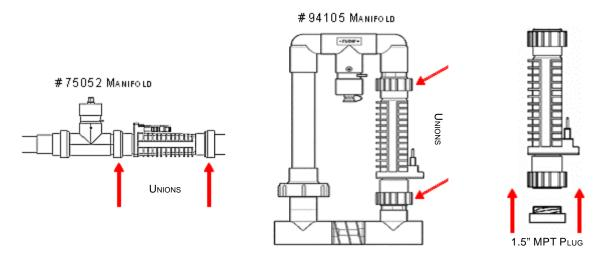
3. Remove the cell and place a cap or plug on the end of the cell as shown. Plugs are available at any pool supply warehouse or home improvement store. Ask for a 1.5" MPT clean out plug.
