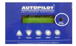
\* Note: When enabled, an audible alarm will sound due to any of the above three (3) conditions. If water flow ceases (or falls below minimum acceptable levels), the alarm will automatically silence after 10-minutes. To enable or disable audible alarm, see "Audible Alarm" programming instructions located on page-30.
