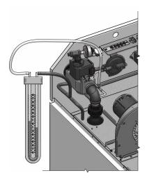
Figure 2-8\_Air Shutter Pressure Measurement
