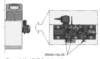
Figure 2-12\_ASME Drain Locations
