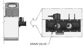
Figure 2-11\_Non-ASME Drain Locations
