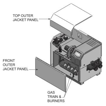
Figure 2-2 Gas Train and Burners
