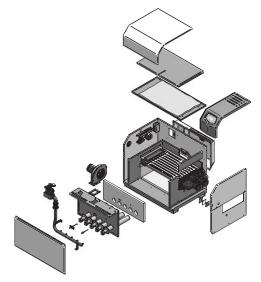
Figure 2-4\_Exploded View of the Heater
