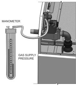
Figure 3-3\_Gas Supply Pressure Measurement - Models ER152 - ER202
