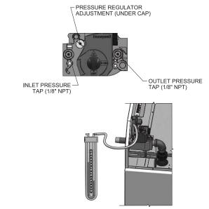
Figure 3-2\_Manifold Gas Pressure Measurement
