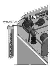
Figure 3-1 Front Chamber Pressure Measurement
