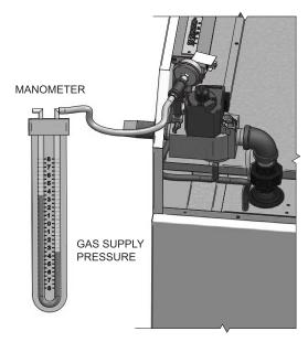
Figure 3-4\_Gas Supply Pressure Measurement - Models ER252 - ER402
