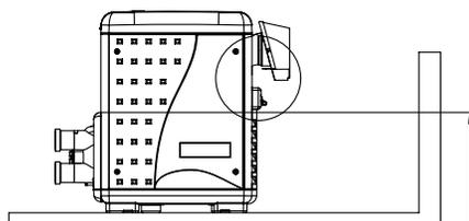
Turn star wheel **counterclockwise** to lower pressure set point if pressure switch is more than 5 feet (1.5M) above water level
