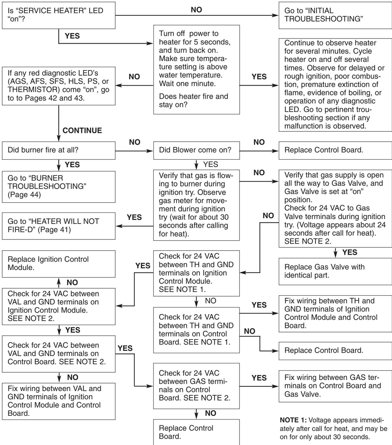
**NOTE 1:** Voltage appears immediately after call for heat, and may be on for only about 30 seconds.
