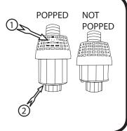
If the valve is NOT popped there is some other problem. Skip to the last step (7) and reinstall the Bypass Valve, Hose Cone and Hose. See Troubleshooting. Section.
