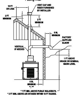
\*USE VERTICAL VENT PIPE TO MEET MINIMUM HEIGHT REQUIREMENTS.
