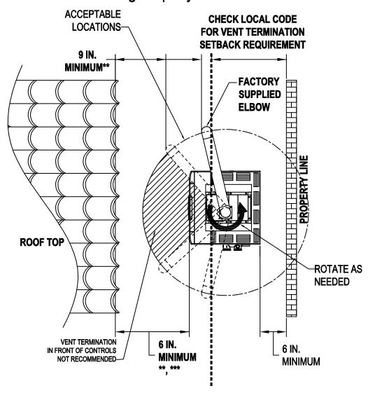
\*USE VERTICAL VENT PIPE TO MEET MINIMUM HEIGHT REQUIREMENTS.
