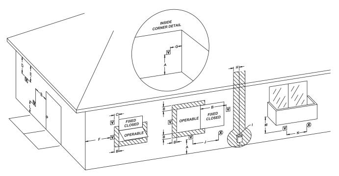
Minimum Clearances from Vent/Air Inlet Terminations—Indoor and Outdoor Installations
