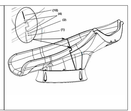
3. Remove the assembled exit and middle slide sections from the pedestal. Turn over and fasten from the underside as shown.
