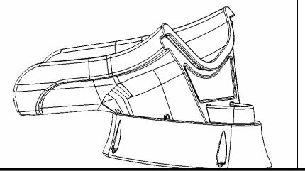
2. Attach the exit slide section to the middle slide section using the hardware shown. If necessary lift up on the exit end to keep the joint tight while fastening.
