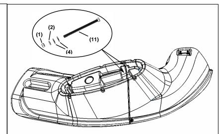
4. Attach the pedestal to the middle and exit slide sections as shown in (3) locations.
