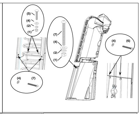
7. Lay the ladder flat and attach the top slide section as shown. Use the appropriate hardware in 4 places. *Note: Use caution not to scratch the ladder during this step!*
