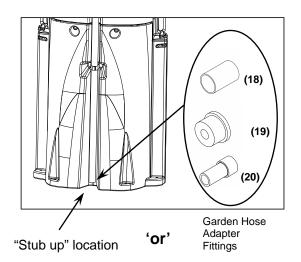
3. Proceed to the following section for **ON-DECK MOUNTING**. After the slide has been mounted to the deck, attach the "stub up" as necessary to the plumbing assembly installed in the ladder.
