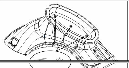
5. Install the 3/8" studs into the threaded inserts in the top of the ladder as shown in (4) locations.
